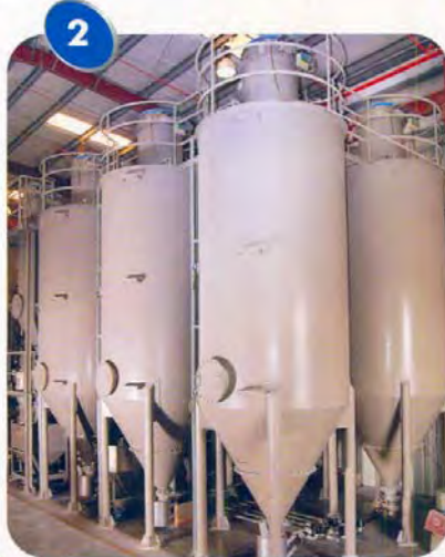
Mixed Materials Storage and Conveying System
